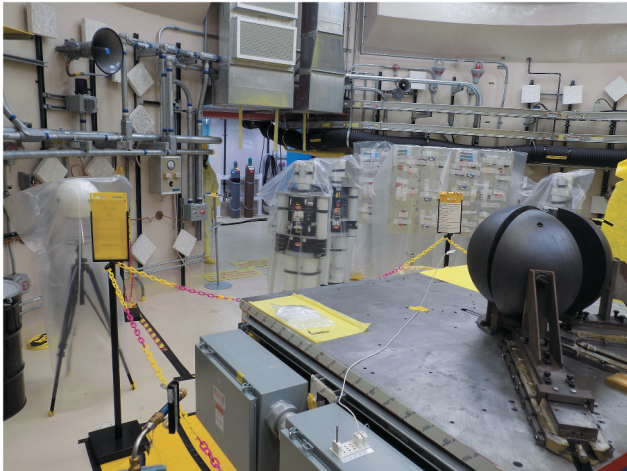
Fig. 18. Dosimetry arranged around flattop for international NAD intercomparison.
